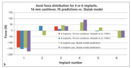
**Fig 16** Vertical forces on 4 or 6 implants supporting a deformable prosthesis with a 8 mm (a) vs. 16 mm (b) cantilever, as predicted using FE methods<sup>16</sup> and the Skalak model. The same trend as seen in Fig 15 is seen here: a more deformable prosthesis does not allow as much load sharing among implants as would be predicted by the Skalak model, which assumes an infinitely rigid prosthesis.
