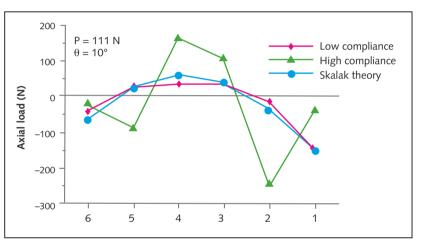
**Fig 13** Results from tests of a system consisting of a loaded rigid steel plate ('prosthesis') supported by load-sensing bolts ('implants') whose axial stiffness values could be adjusted<sup>9</sup>. The plate is loaded by 111 N at a cantilever position distal to implant no. 1. Results from Skalak calculations are not shown for the 'High compliance' case; see reference <sup>9</sup> for this detail.
