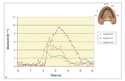
**Fig 18** Example of *in vivo* forces and moments on implant abutments supporting a metal prosthesis in a patient who is asked to open his jaw at about the 1-s mark in the plots; vertical force components occur (tensile and compressive, depending on the implant) as well as bending moments<sup>31,34</sup>.
